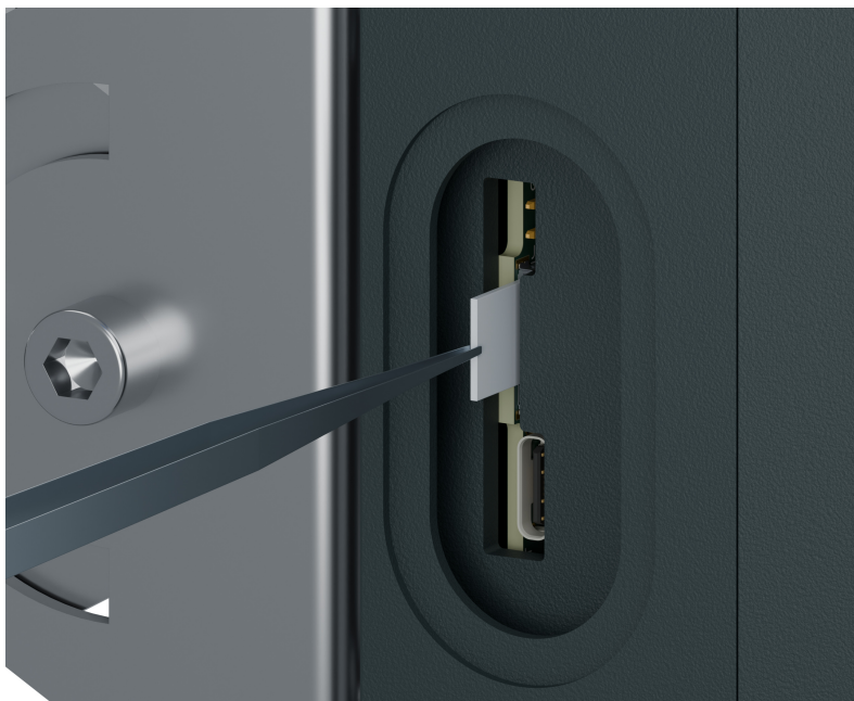
Remove and insert the SIM card
